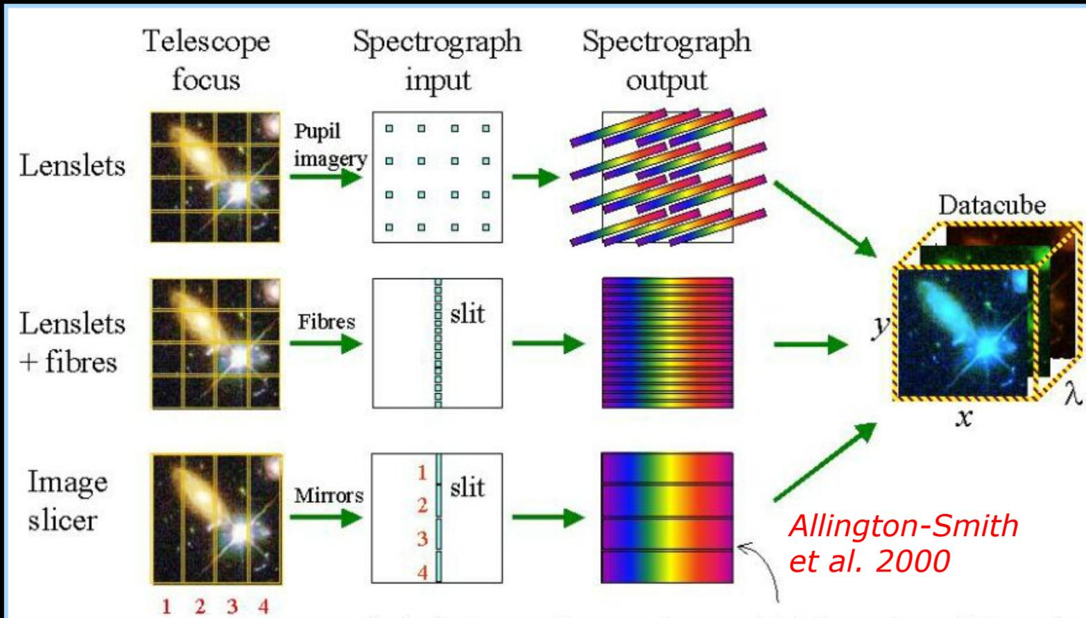
Records simultaneously three variables ( $\alpha$ ,  $\beta$  and  $\lambda$ ) in two dimensions ( $x$  and  $y$ )
