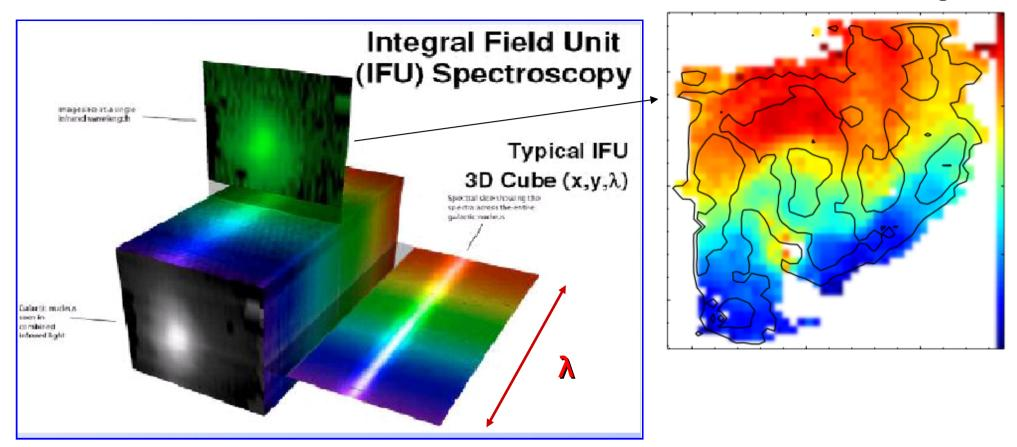
Finally a 3D cube containing SPATIAL (x, y) & SPECTRAL information is produced!
